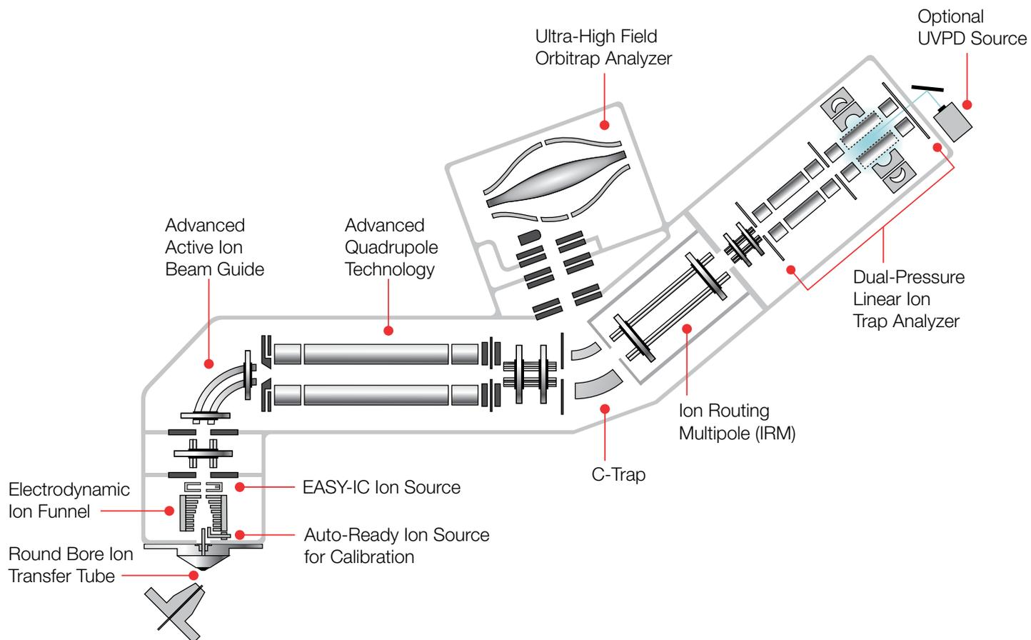
Figure 2. Orbitrap IQ-X Tribrid mass spectrometer schematic.
